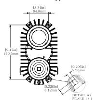
Mounting tabs sized for M5 or #10 fasteners.
