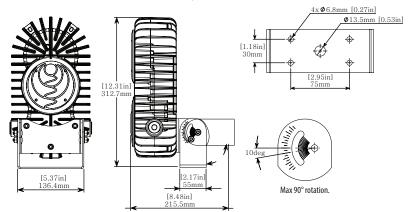
Mounting holes sized for M6 or 1/4" fasteners.
